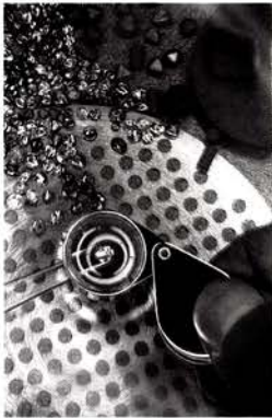
Natural diamonds used in drill bits are graded for size and quality before being mounted in a bit.
