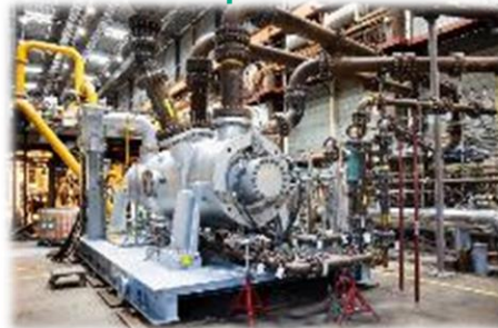
Compression train undergoing testing at our Le Creusot facility in France
