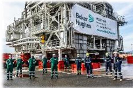
Turbomachinery equipment packaged with electric generators, waste heat recovery system and auxiliaries into an industrial module ready to ship at Avenza, Italy
