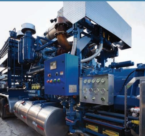
*In 2012, Baker Hughes introduced bifuel pumps into some of our U.S. hydraulic fracturing fleets. Using natural gas to reduce diesel use by up to 65% meets all U.S. emissions standards, requires less fuel, and improves job site safety by reducing refueling during pumping operations.*
